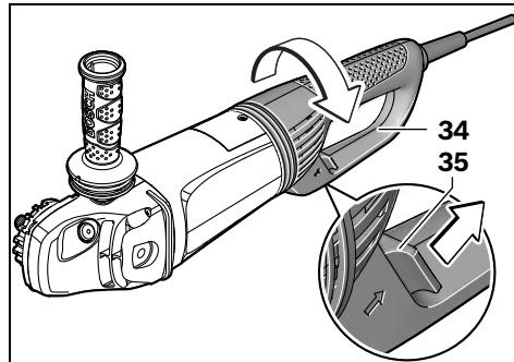
The main handle 34 can be rotated with respect to the machine housing toward the left or right in steps of 90°. In this manner, the On/Off switch can be brought into a more convenient position for special working situations, e.g., for cutting operations using the cutting guide with dust extraction protection guard 18 or for left-handed persons.
