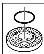
A plastic part (O-ring) is fitted around the centring collar of mounting flange **5**. **If the O-ring is missing or damaged,** the mounting flange **5** must be replaced before resuming operation.
