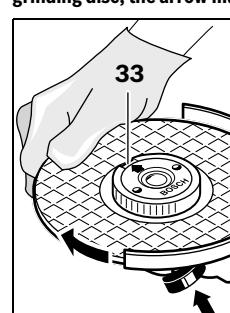
Lock the grinder spindle with the spindle lock button 1. To tighten the quick-clamping nut, firmly turn the grinding disc in clockwise direction.
