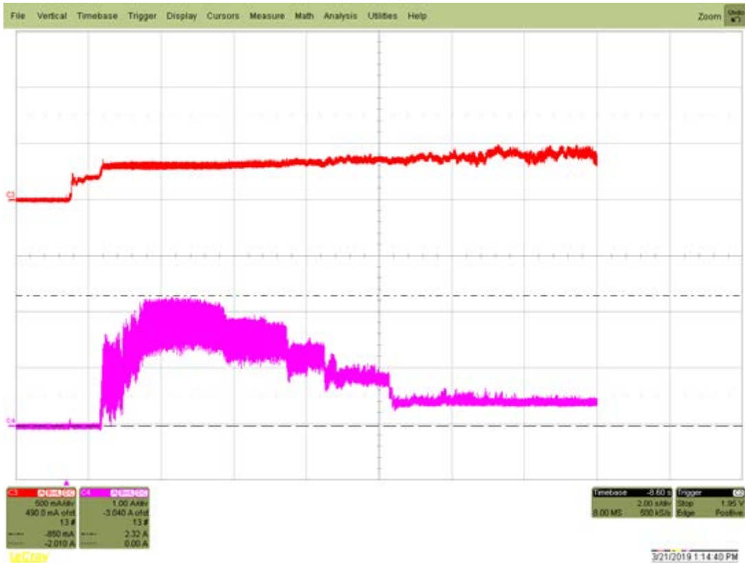
Figure 3. 4TB Typical startup and operation current profile
