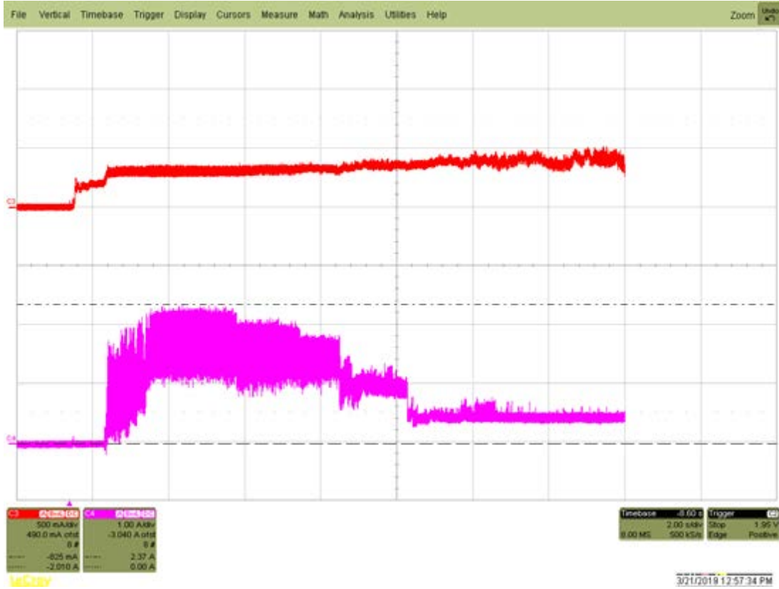
Figure 1. 8TB Typical startup and operation current profile
