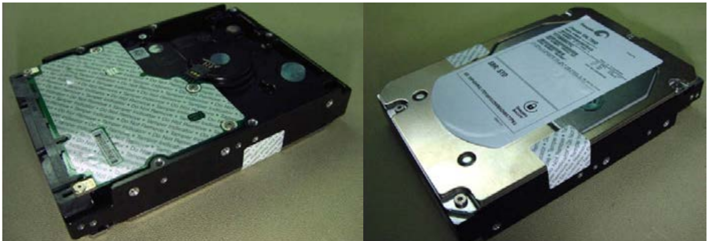
Figure 9. Example of FIPS tamper evidence labels.
