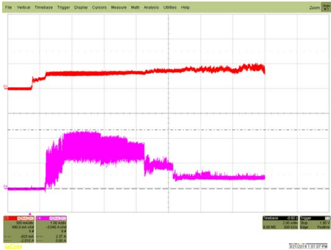
Figure 2. 6TB Typical startup and operation current profile
