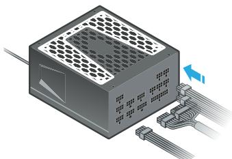
**4.4.** Connect all the necessary system DC cables (Motherboard, CPU, VGA, HDD, Optical Drivers, etc). The connectors should click to lock in.
