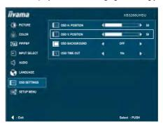
Press the ◀ Button lastly to close the On Screen Display feature. All changes are saved in the memory.
