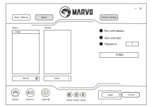
And then click "Stop" to end recording process. Execute a macro, such as the mouse button "4" key set to "macro", press the mouse "4" key to play the recorded content.
