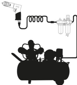
All control elements, connecting lines and hoses should be intended for the necessary pressure and the air flow rate. Do not allow the narrowing of feeding lines, for example, as a result of cross-clamping, bending, or stretching. Before connecting a hose to the tool, regularly blow the hose with a strong air stream to remove moisture from the hose.
