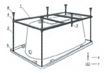
3. Install the stud (2) in the frame opening, screw the stud onto the plastic supports (5).
