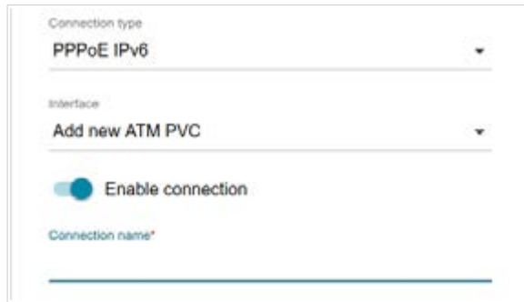
Figure 63. The page for creating a new PPPoE IPv6 connection. Selecting a connection type.
