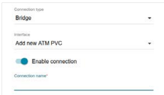
Figure 70. The page for creating a new Bridge connection. Selecting a connection type.
