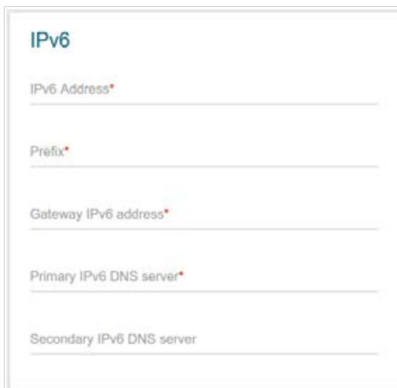
Figure 54. The page for creating a new Static IPv6 connection. The IPv6 section.
