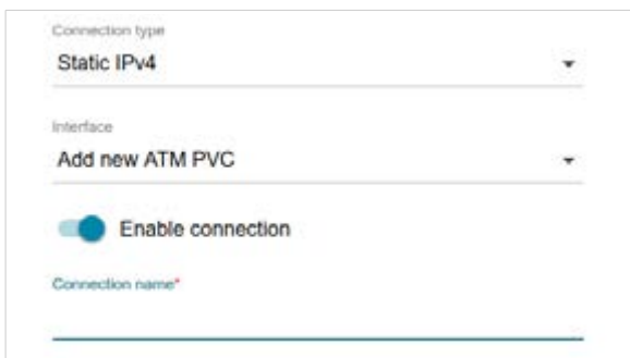
Figure 45. The page for creating a new Static IPv4 connection. Selecting a connection type.
