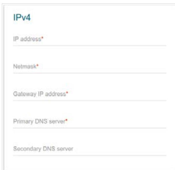
Figure 48. The page for creating a new Static IPv4 connection. The IPv4 section.
