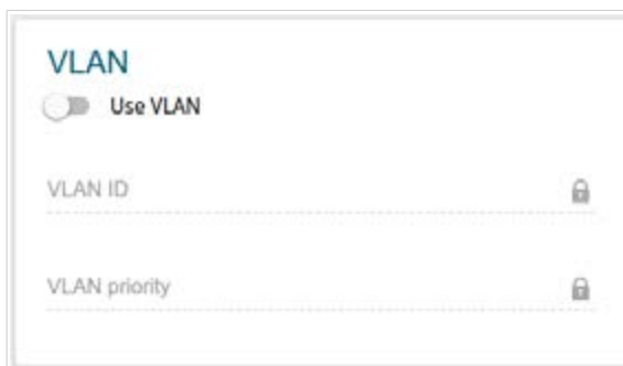
Figure 69. The page for creating a new PPPoE IPv6 connection. The VLAN section.
