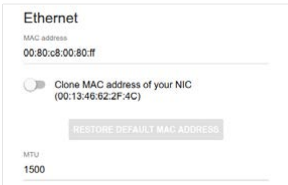
Figure 64. The page for creating a new PPPoE IPv6 connection. The Ethernet section.
