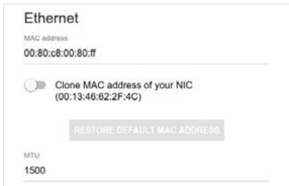
Figure 52. The page for creating a new Static IPv6 connection. The Ethernet section.
