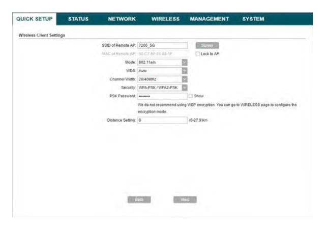
**6.** Create a new *SSID* and *PSK Password* for the local wireless network. The wireless AP settings for the local network will be set the same as your root AP by default. Click **Next**.
