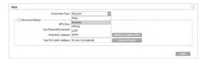
There are five WAN connection types: Static, Dynamic, PPPoE, L2TP, and PPTP. Select the suitable one to configure the IP parameters of the WAN on the screen below. If you are not sure of the connection type, please consult your ISP.
