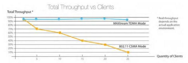
Pharos MAXtream is a proprietary protocol developed on the basis of TDMA (Time Division Multiple Access) by TP-Link. MAXtream cuts each wireless data frame transmission into certain number of time slots according to the client connections priority, greatly boosting efficiency of the wireless channel.
