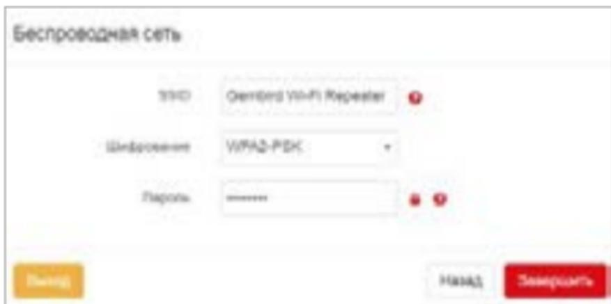
The screenshot shows a web interface titled "Беспроводная сеть" (Wireless network). It contains three input fields: "Имя" (Name) with the value "Gembird Wi-Fi Repeater", "Шифрование" (Encryption) with the value "WPA2-PSK", and "Пароль" (Password) with masked characters "\*\*\*\*\*". There are red error icons next to the Name and Password fields. At the bottom, there are three buttons: "Отмена" (Cancel), "Назад" (Back), and "Завершить" (Finish).
