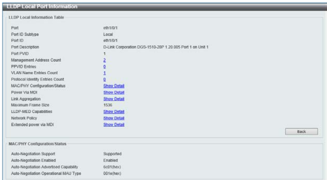
Figure 5-69 LLDP Local Port Information - Show Detail window
