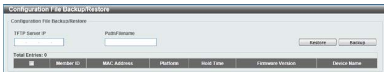
Figure 4-72 Configuration File Backup/Restore window
