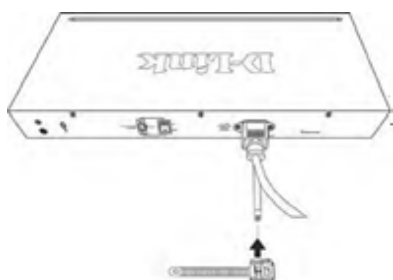
Figure 3-3. Slide the Retainer through the Tie Wrap
