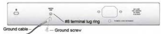
Figure 2. Connect a Grounding Cable
