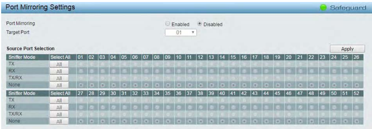
Figure 4.52 – L2 Functions > Port Mirroring
