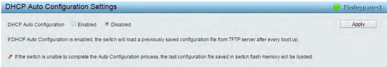
Figure 4.27 – System > DHCP Auto Configuration
