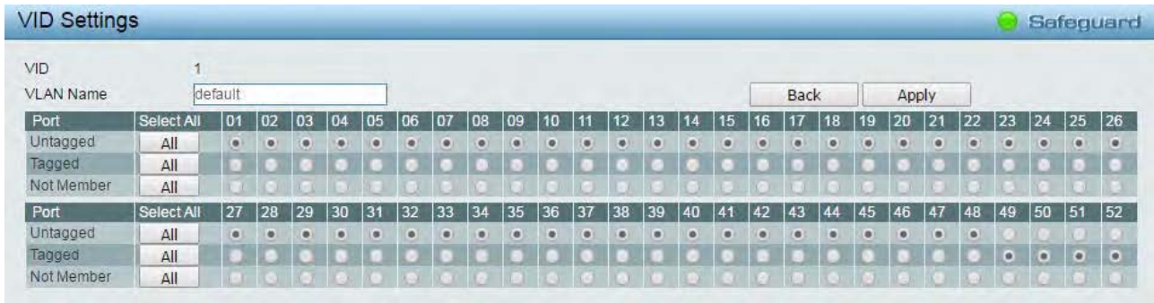
Figure 4.42 - Configuration > 802.1Q VLAN > VID Assignments
