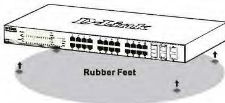
Figure 2.1 – Attach the adhesive rubber pads to the bottom
