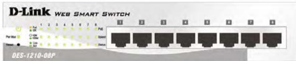
Figure 1.1 – DES-1210-08P Front Panel
