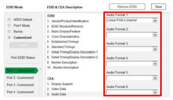
Use the drop down menu to select the **Audio Format** ( $1\sim6$ ) applicable to your audio output device, and click **Save** to apply the changes.
