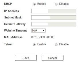
**Enable** DHCP to allow the DHCP server to assign an IP address to the VM6404H / VM6809H. Select **Disable** to enter your own static IP address settings for the device.
