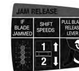
If blade jammed all fuel gauge LEDs will blink.
