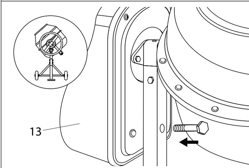
Turn the drum, as shown in the figure, install the bolt M8 x 55 and the washer, pos. 8 to fasten the drive.
