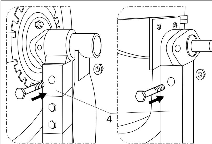
Install the bolts M8 x65 and fix the cross beam supports on the frame, pos. 4 with nuts M8, as shown in the figure.
