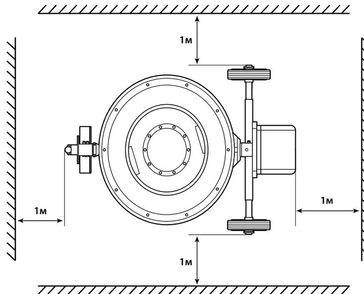
The mixer operates in cycles with the following sequence: loading, mixing, unloading. The mixer should be installed on a plain and solid horizontal surface. It is recommended to turn on the mixer with the drum in a vertical position.
