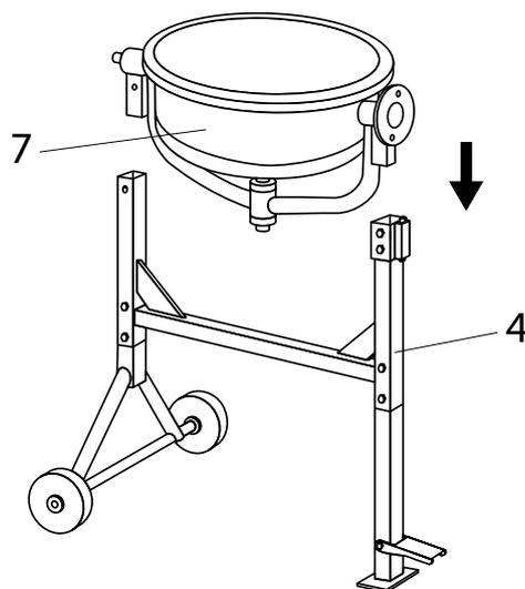
Install the lower drum with a cross beam, pos. 7 on the frame, pos. 4. The installation should be carried out by two persons.
