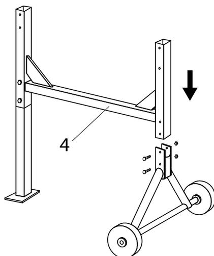
Connect the wheel support complete with the frame, pos. 4 by means of bolts M8 x 65 and fix with M8 nuts.
