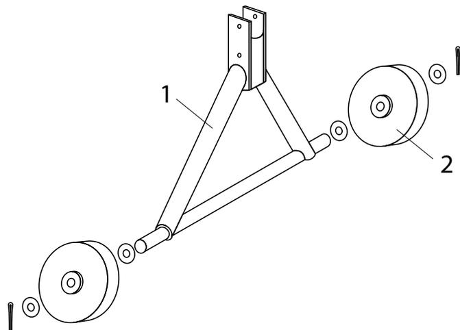
Set on the wheel support axis, pos. 1 washer 27, then wheel, pos. 2 and one more washer 27. Insert into axis openings the splints so that they are located at the outside of the washer. Remove splints, using flat-nose pliers..
