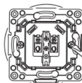
Install the mechanism into the hollow in the wall, tighten firmly the locking and the fastening screws on the unit housing.
