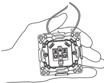
Connect the wires by pushing the skinned ends into the grooves of terminals clamps. If there is a grounding wire, connect it to the appropriate contact. Tighten the screws.
