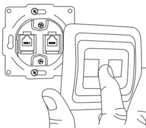
Install the mechanism into the hollow in the wall, tighten firmly the locking and the fastening screws on the unit housing. Install the decorative frame and the cover.
