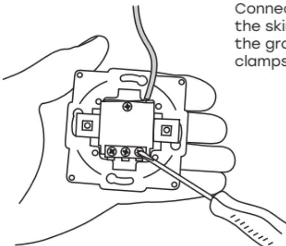
Connect the wires by pushing the skinners (Fig. 3.1.) into the grooves of terminals clamps and tighten the screws.
