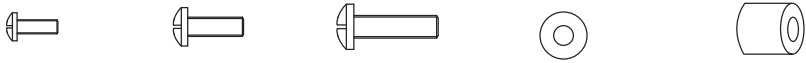
(A) M4x25 screws (4) (B) M5x25 screws (4) (C) M6x25 screws (4) (D) \Phi 6 Flat washer (4) (E) 12mm Plastic Sleeve (4)
