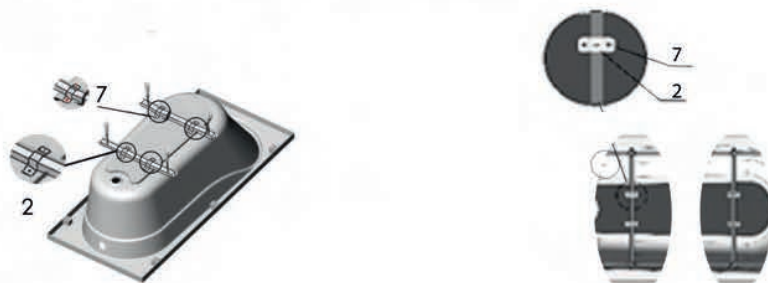
Pic.5 bath legs fixation
