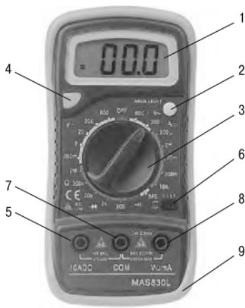
1 – 3 ½ digits LCD, height of characters 12.7 mm. Display shows measurement results in digital form.
