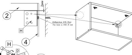
Монтаж задней стенки Installation of the rear wall of the
