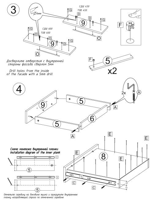
Mark the middle on the side of the drawer and screw the inner rail in exactly the marked middle
