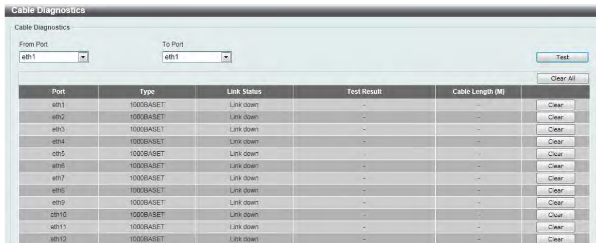
Figure 10-1 Cable Diagnostics window
