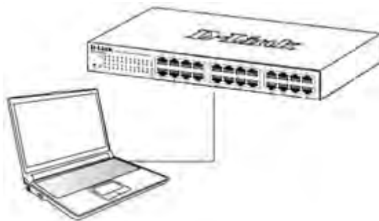
Figure 4-1 Connecting to a DGS-1100 Series Switch
