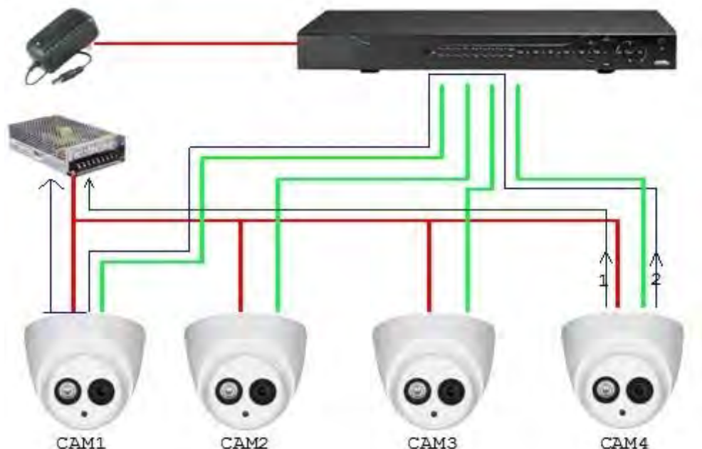
Figure 10-1 Principle of centralized power supply
