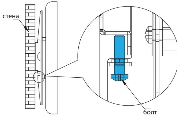
EN Fix the two bolts under the monitor brackets inside of the wall plate and then screw them down.
