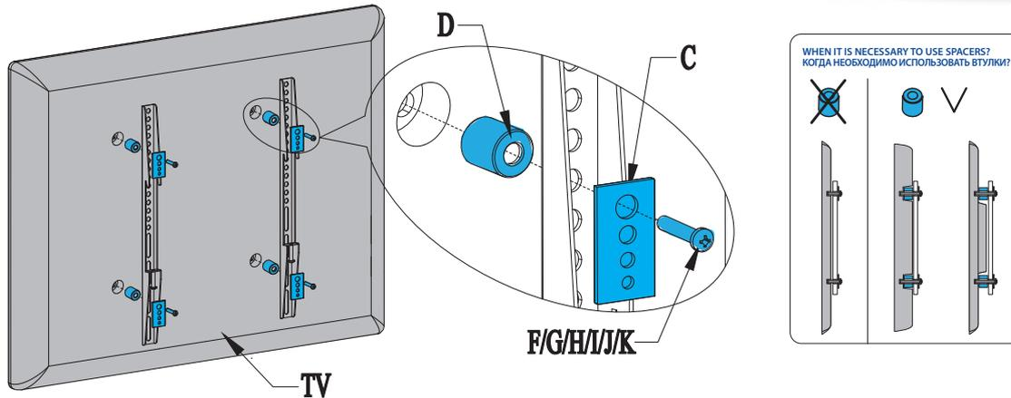
**EN** Select the suitable bolts from the parts bag according to the TV size and the thread holes at the back of TV. Screw 4 selected bolts (F,G,H,I,J,K) into the thread holes on the TV back through washer (C) and the corresponding holes on the monitor bracket. Make sure the distance from each bracket to the top of the panel TV is equal, and also as center as possible. The bolts should be screwed down. Don't tighten the screws too hard
