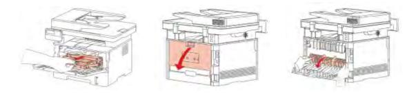
**Step2:** Gently pull the jammed paper out, then c lose the back cover after removing the paper jammed, install a new toner cartridge and then close the front cover; then, the printer will recover printing automatically.
