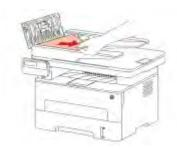
**Step2:** After removing the paper jammed, close the top cover and then the printer will be back to the ready state. If it is difficult to remove the paper jammed, please try to open the scanner cover and remove it from the pressing block.
