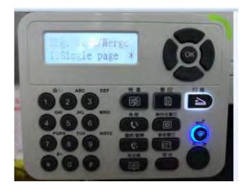
Step 2: Press "▲" or "▼" button to select and enter "Merge Scan" mode.
