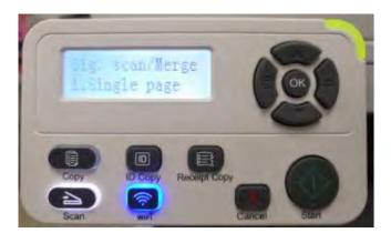
Step 2: Press "▲" or "▼" button to select and enter "Merge Scan" mode.
