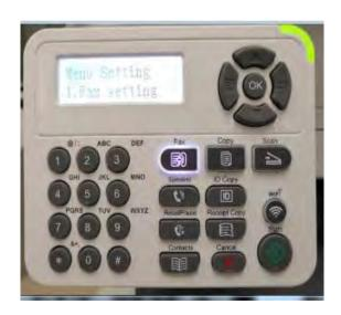
**Step4:** Enter the fax number one by one by pressing the number on the control panel.
