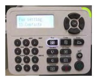
**Step4:** Enter the fax number one by one by pressing the number on the "NO.4 New and edit"
