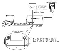
Refer to the steps below to mount the Switch on a Wall.
