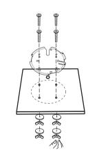
Secure the mounting bracket to the ceiling tile using four M3x30 pan-head screws, washers, and wing nuts, as shown on the left.
