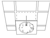
Feed the Ethernet cable through the hole and set the ceiling tile back into place.
