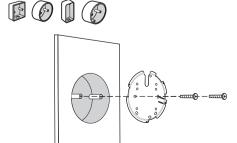
Route the cables through the square cable hole on the mounting bracket, and secure the mounting bracket to the junction box using screws. Then follow Step 4 and Step 5 of Option 2 to complete the installation.
