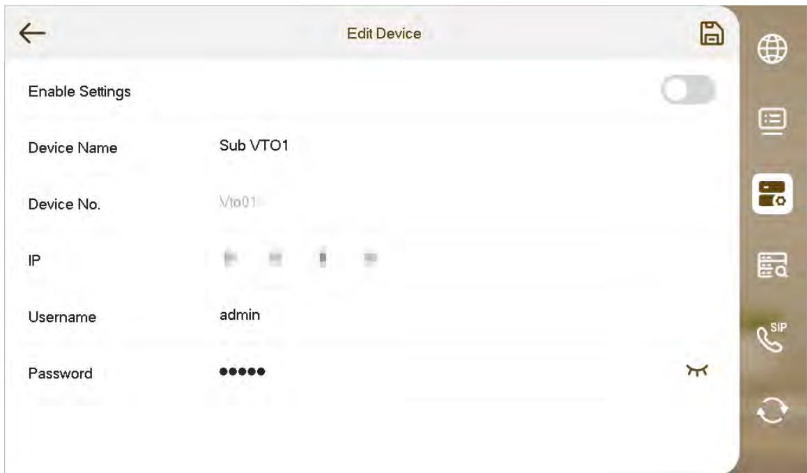
Figure 3-53 Sub VTO configuration
