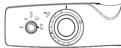
Other example. Wheel D has been turned to a position corresponding to 21 °C. The thermometer displays a temperature value of 18 °C. Consequently, the calibration value is –3 °C (three divisions).
