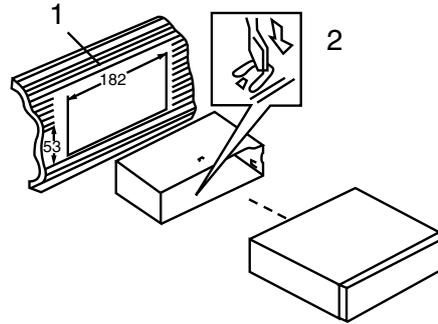
1. Install the sleeve into the dashboard; ensure it is installed with the correct side and there are no obstacles (wires, dashboard elements, etc) for the unit installation.
