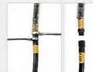
Disassemble & replace the connection air hose.
