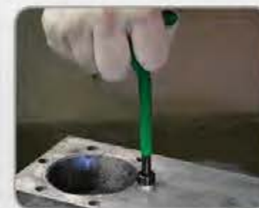
4. Screw coil into casting
