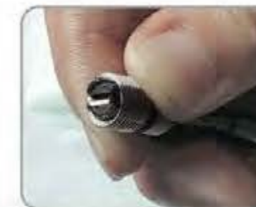
3. Load coiled insert into applicator
