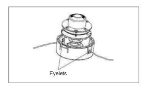
Align the protrusion on the underside of the cover with the slots of the eyelets.
