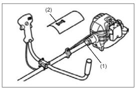
Insert the throttle cable (1) of control lever into the clamping slot (3) of lower splint of handle holder.
