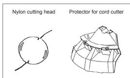
CAUTION: The appropriate protector must always be installed, for your own safety and in order to comply with accident-prevention regulations. Operation of the equipment without the guard being in place is not permitted.
