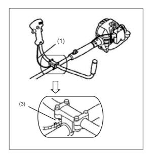
CAUTION: After waist pad is packed, the redundant throttle cable close to the engine side can not be curved which can cause phenomenon of too high idle speed and the blade can not stop, see right photo.
