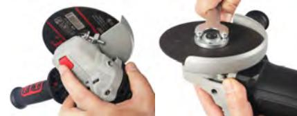
Lock the grinding spindle with the spindle lock button before clamping and releasing the abrasive tools.
