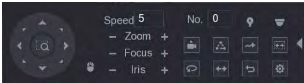
Figure 5-69 Expanded PTZ control panel
