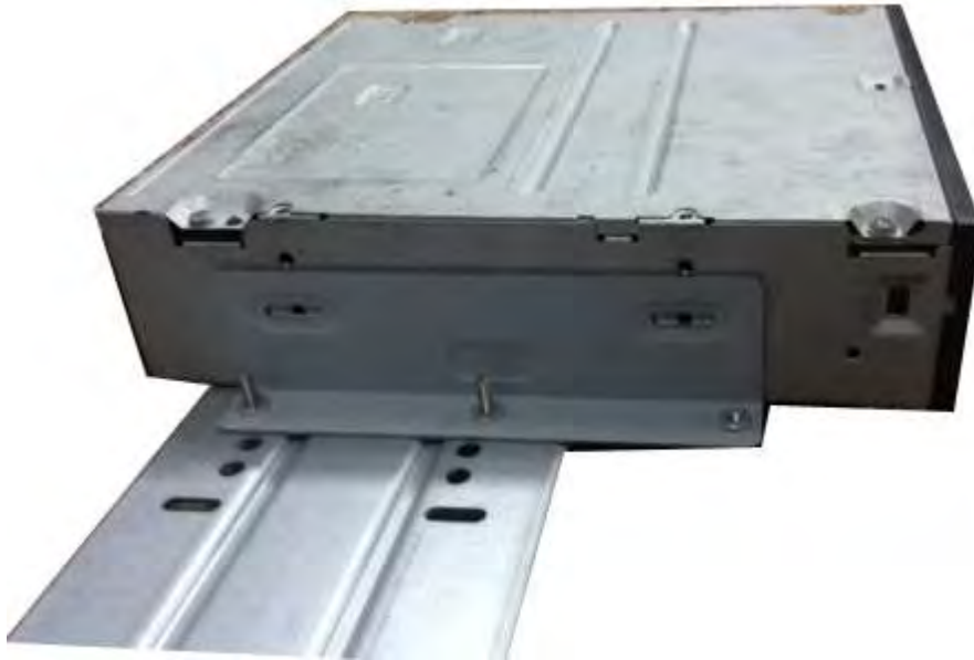
Figure 3-43 Install SATA burner
