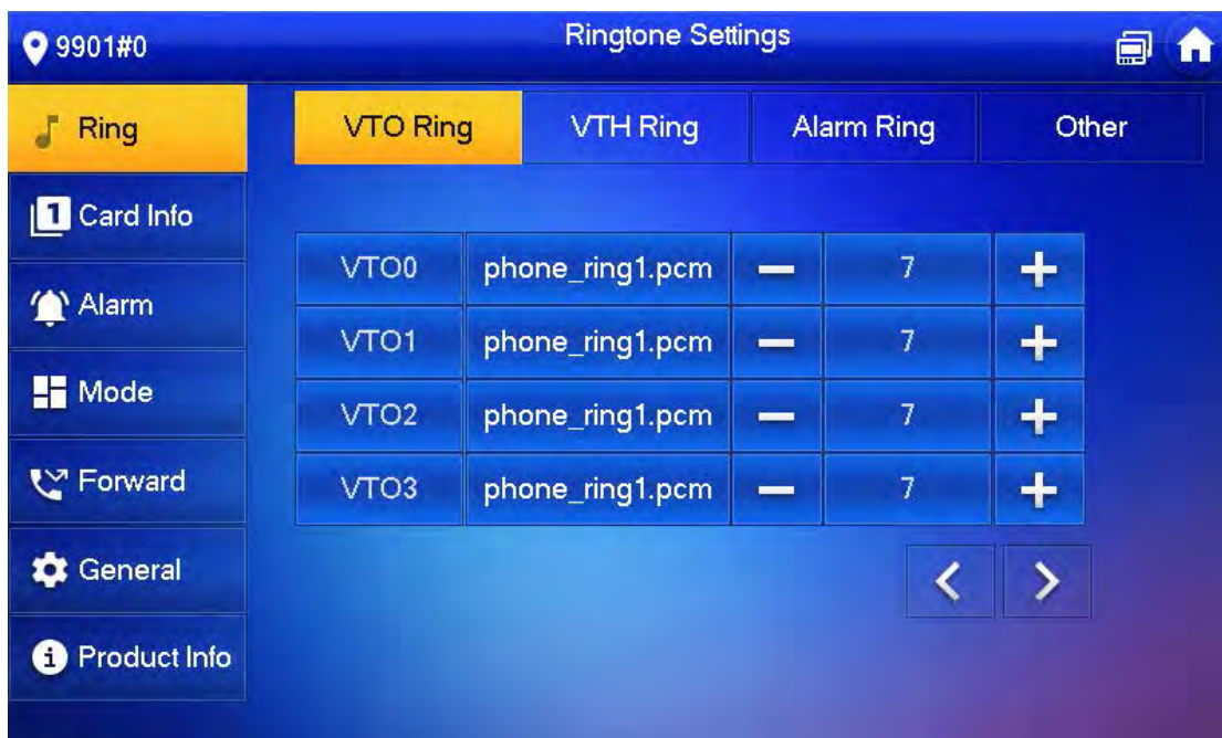
Figure 4-22 VTO ring setup
