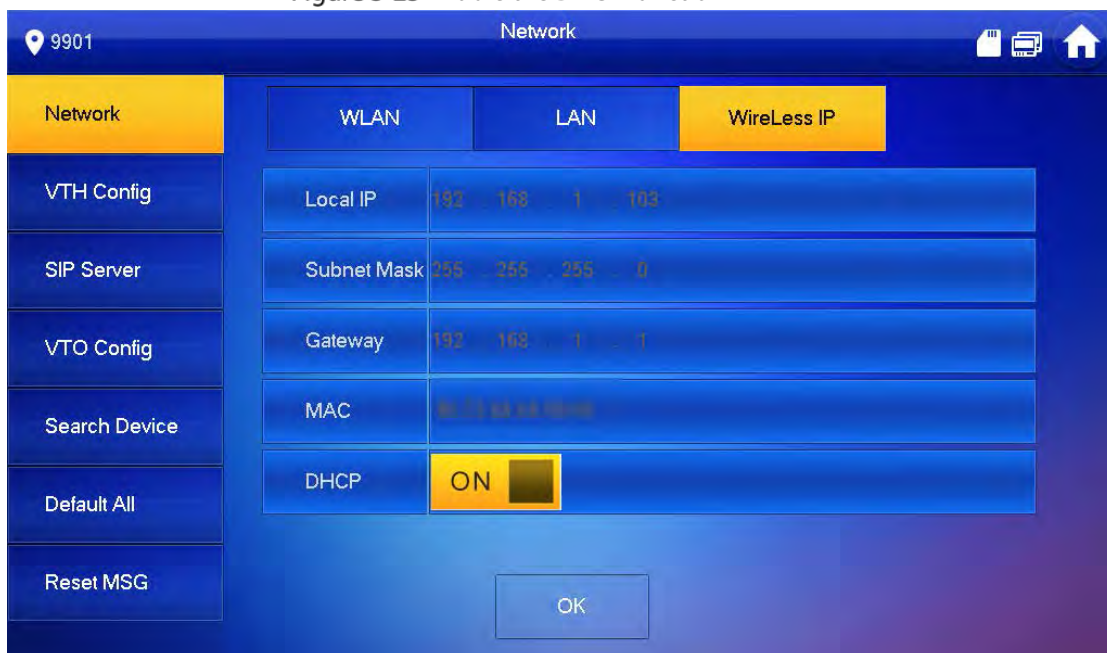
Figure 3-25 Enable the DHCP function
