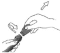
Figure 3-23: Unscrewing the microphone head grille
