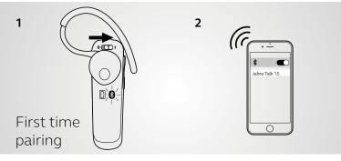
1. Slide the On/Off switch to On. The Bluetooth LED will flash blue.
