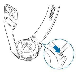
2 Slide the spring bar inwards and connect the band.
