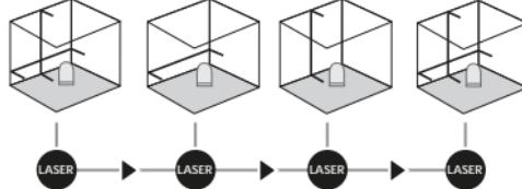
**!** The transport restraint must be released for horizontal and vertical levelling. The LED shows a permanent green light. The laser lines flash and the LED lights red as soon as the device is outside the automatic levelling range of 5°. Position the device such that it is within the levelling range. The LED switches back to green and the laser lines stop flashing (steady light).
