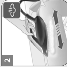
EN Figure 2: Slower movement, less steam. Figure 3: Faster movement, more steam.
