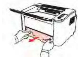
**Step2:** Paper Jam around fuser unit the Printer, Open the upper fuser guide to decrease the pressure of compression spring, Pull the jammed paper out of the fuser unit.
