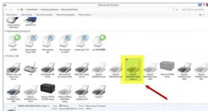
**Step3:** Click PC table “start”-“printer and fax”, chose any of the printer copy, the mouse right click on the “printer property”--“port”, then chose the customer no need the printer copy port of all the printers, and click "delete port"-“confirm”. At last reconnect to the printer and re-install the driver.
