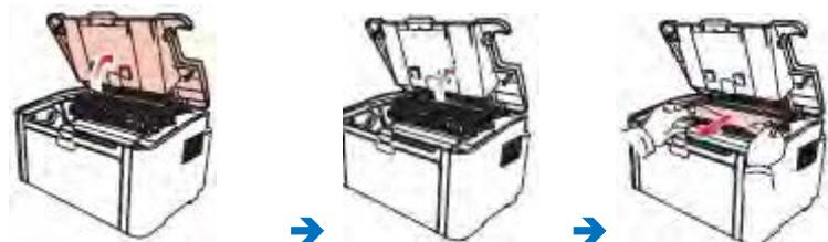
**Step3:** Paper jam inside the printer. Remove the laser toner cartridge along the guides, slowly pull the jammed paper out along the paper output orientation, and then insert the laser toner cartridge into the printer.
