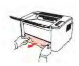
**Step2:** Paper Jam around fuser unit the Printer, Open the upper fuser guide to decrease the pressure of compression spring, Pull the jammed paper out of the fuser unit.
