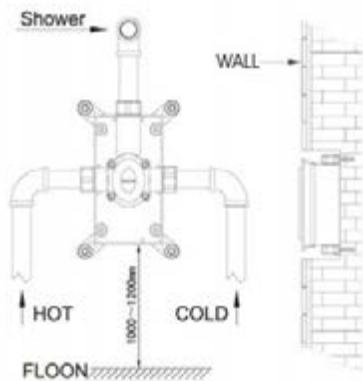
Provide the dimension of the in wall box for drilling. Fixed the in wall box by exploded screw.
