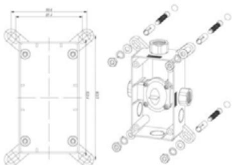
Connect the hot, cold and outlet pipe. Open water switch to check if each joint is tight, no leakage and no crack. After using proper pull and push, the wall could be covered with tile.
