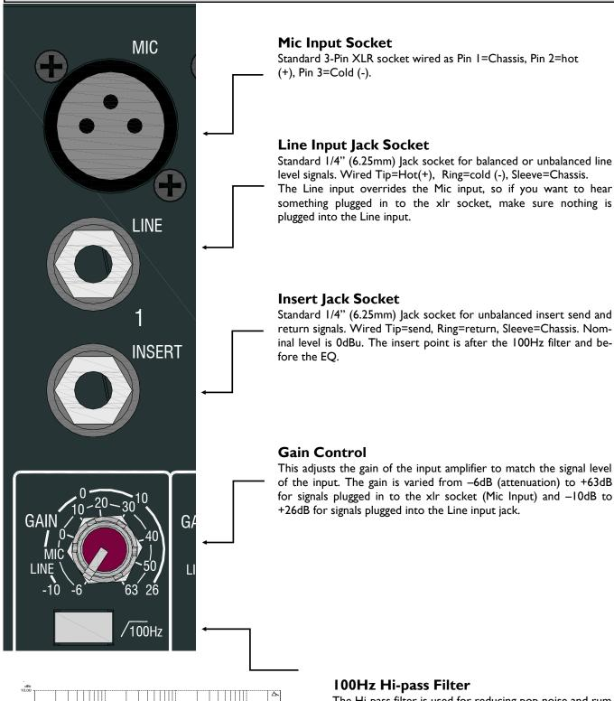
The Hi-pass filter is used for reducing pop noise and rumble from microphone signals. It is a 2-pole (12dB per octave) filter with a corner frequency set at 100Hz.
