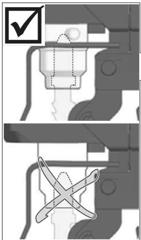
Press the saw blade into the Fixtec holder up to the stop.
