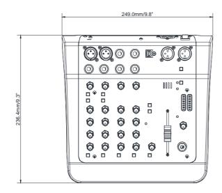
HEIGHT: 88.9mm (3.5") WIDTH: 249mm (9.8") DEPTH: 236.4mm (9.3")
